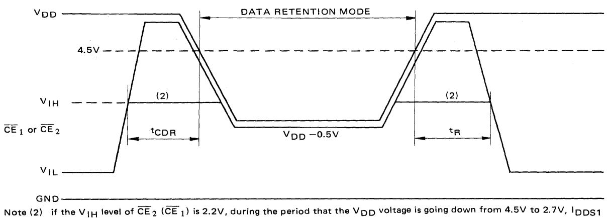
Note (2) if the  $V_{IH}$  level of  $\overline{CE}_2$  ( $\overline{CE}_1$ ) is 2.2V, during the period that the  $V_{DD}$  voltage is going down from 4.5V to 2.7V,  $I_{DDS1}$  current flows.
